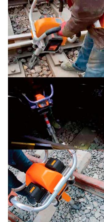
Lithium battery cutting machine AJL- LDC2001
