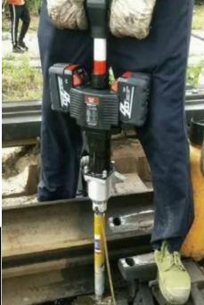
Lithium battery rail drilling machine AJL- LDZ1501
