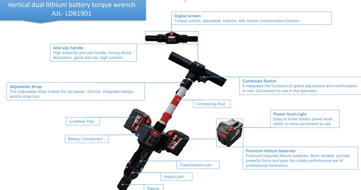
Vertical dual lithium battery torque wrench(model :AJL- LDB1901) vertical operation Railway digital torque wrench with dual lithium battery protection technology. Its working torque > 3000N.m, torque can be adjusted and controlled, professional for railway bolting operations.
